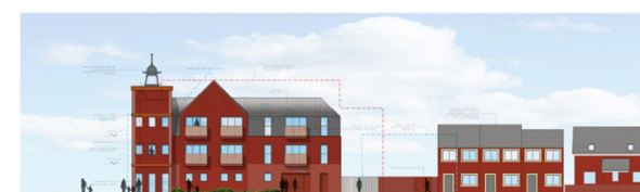
2018 Planning Design (large gable as per chapel, square tower with retained bell, roof form steps down)
